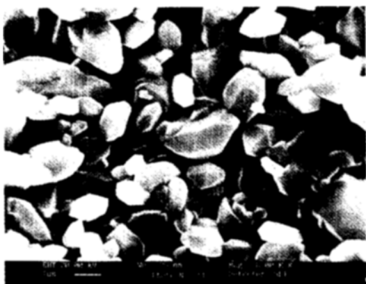
Fig. 9. SEM micrograph of \alpha -quartz powders formed with 1.5 wt% NaF (reaction time: 3 h, seed=0.5 wt%, at 400°C).
