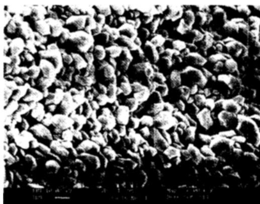
Fig. 5. SEM micrograph of \alpha -quartz powder formed with 0.075 wt% KOH (reaction time: 3 h, seed=0.5 wt%, at 400°C).
